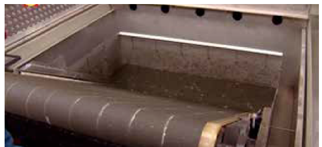
Filters are installed in channels and have integrated dewatering.
